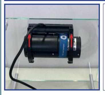
Adjustable mount - The forward facing camera is placed in the mount with the wire protruding out the top of the camera and the back of the mount is hinged up to hold the camera and then secured in place using a T10 torx key.
