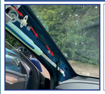
After the molex connector is connected the cable routing can take place.
