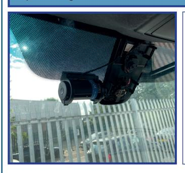
After cleaning the selected area with the wipe you are ready to mount the camera ensuring the best placement for the type of vehicle, remove the red film backing from the mount, then pressing the mount gently onto the windscreen to ensure a firm adhesion to the windscreen, this can be checked by looking at the mount from the outside.
